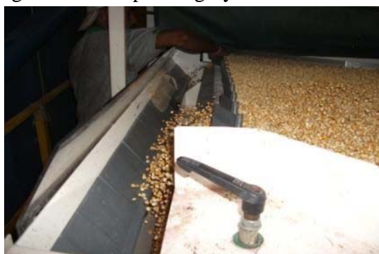
Picture.8 The gravity machine for separating by weight of seeds
